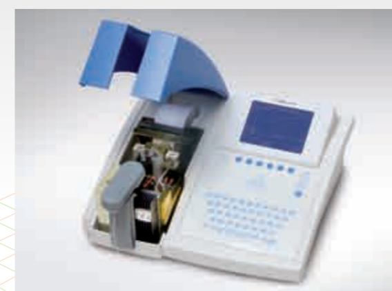
Microlab 300 with open service cover
